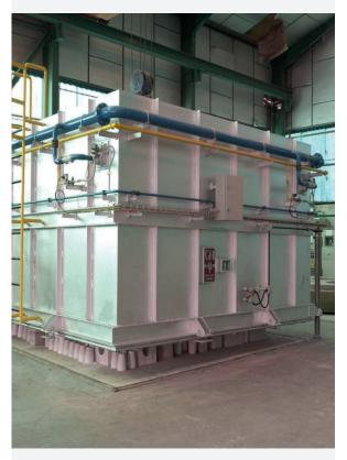
For the heat treatment of steels, maintained temperatures of approximately 900°C are required, in addition to outdoor cooling at room temperature.
